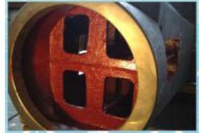
COLUMN: box structure, increase rigidity
